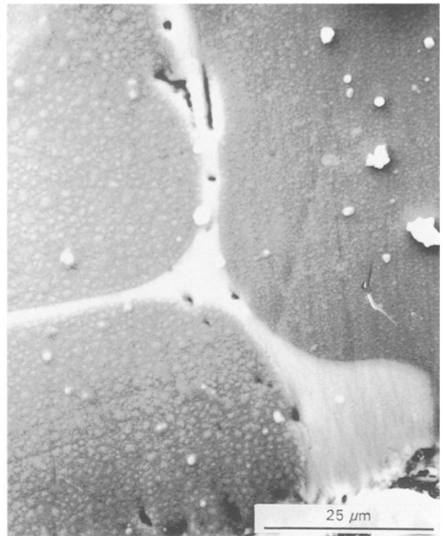
Figure 3 Micrograph of a sample B showing second phase containing calcium and silicon.
